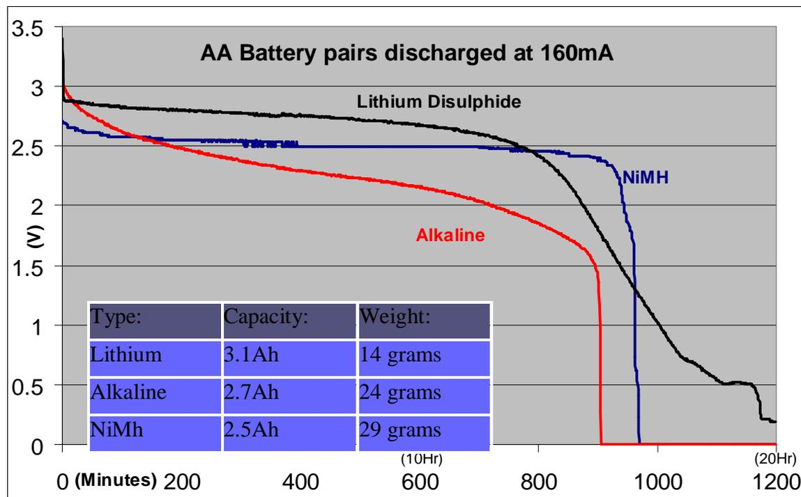
The above graph shows the discharge rates of the typical battery options. It shows that the Lithium and 2500mAh NiMh can significantly outperform even the best alkaline batteries.
