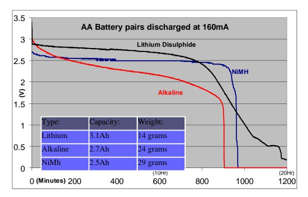
The above graph shows the discharge rates of the typical battery options. It shows that the Lithium and 2500mAh NiMh can significantly outperform even the best alkaline batteries.
