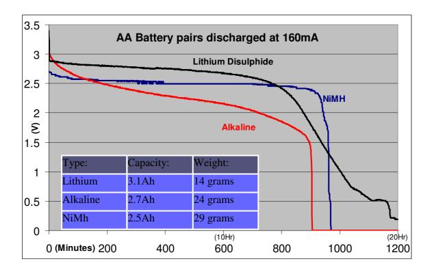
The above graph shows the discharge rates of the typical battery options. It shows that the single use Lithium and 2500mAh NiMh can significantly outperform even the best alkaline batteries. New low self discharge offerings like the Panasonic "Eneloop" or Eveready "Recharge Extreme" can be considered if you use the sniffer regularly wish to save money in the long run.
