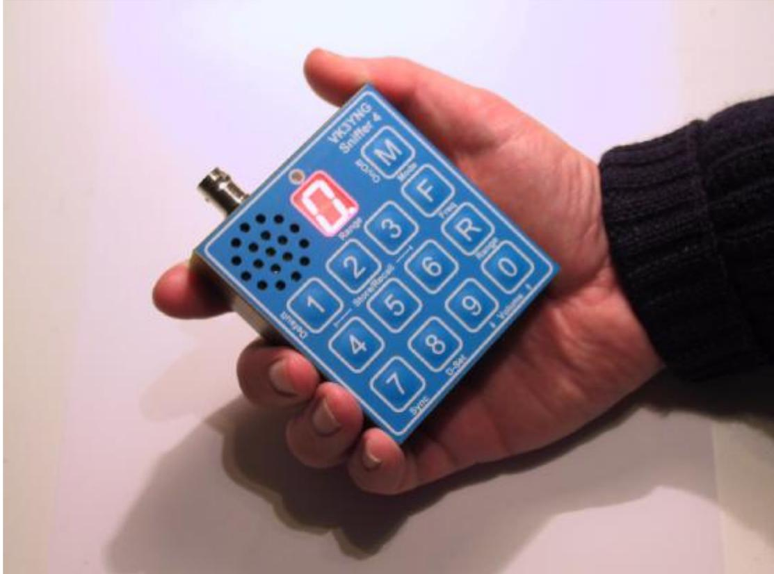
The VK3YNG Foxhunt Sniffer is a specially designed synthesised VHF direction finding receiver covering 120MHz and 144MHz bands.
